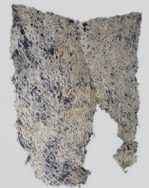
Paper making from Ravenala tree and Bagasse
