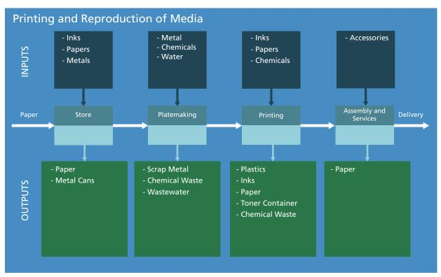
Figure 26: Process flow diagram for the printing and reproduction of media industry
