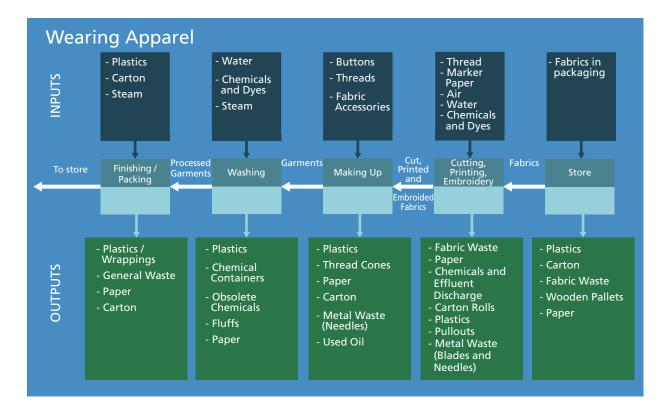
Figure 22: Process flow diagram for the wearing apparel industry
